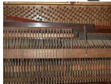
The hammers are underneath a 'shelf'. If you take the front off the piano there are stiff wires at the front of the action
