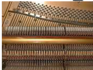
You can clearly see the hammers when they hit the strings
